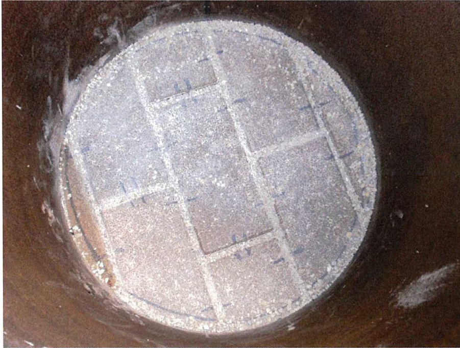
Figure 4 4x8 Permeable 2-1/4" Beveled Paver After Compaction
