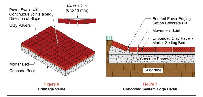
drains can be incorporated in the middle of large paving systems and can be installed to drain water that has penetrated the mortar bed. Gutters and swales (see Figure 6) can be formed by slightly dishing or recessing the pavers in the mortar setting bed. Suspended structural slabs often incorporate a drainage mat under the mortar bed to allow the water to drain out at that level. To aid drainage, continuous joints should be aligned with the direction of water flow.
