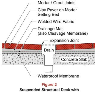
Suspended Structural Deck with Unbonded Mortar Set Paver System
