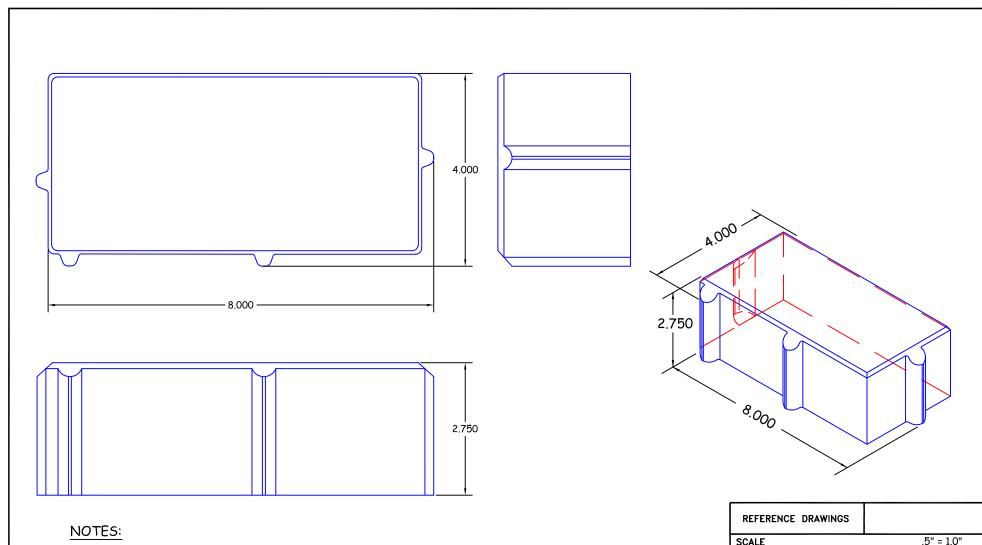
Complies with ASTM C1272 Type R Application PS Application PX available on request
